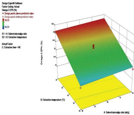
Figure 2. Effect of extraction temperature and solvent:algae ratio on the omega-3 EPA content.
