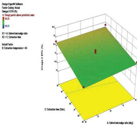
Figure 3. Effect of extraction time and solvent:algae ratio on the omega-3 EPA content.
