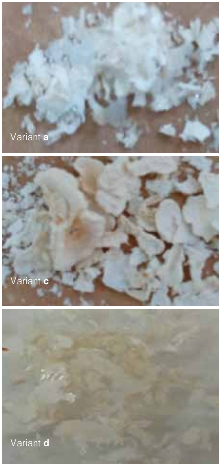
Figure 1. Pectin extracts obtained from carrot pulp by enzymatic (a), thermal (c) and microwave-assisted (d) methods
