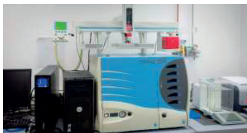
Figure 2. A-Prometheus Multisensor System (E-nose)
