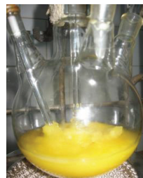
Figure 3. Cold saponification of vegetable oils using a laboratory glass installation
