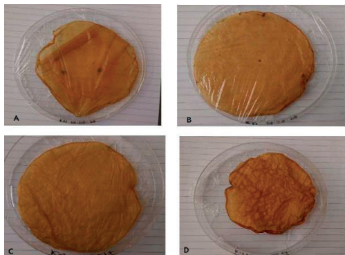
Figure 2. Aspects of Kombucha biofilms dried during 18 days at 35°C (A: black tea; B: oolong tea; C: green tea; D: green tea + Melissa officinalis )
