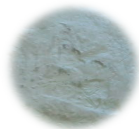
Figure 1. Sponge biomaterial based on fish collagen mixed with chitosan solution, pH 5 in 1:1 weight ratio
