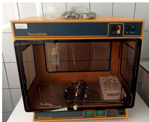
Figure 3. The thermoshaker for incubation of transformed cells
