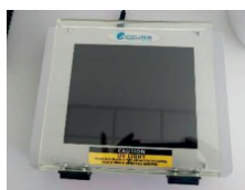
Figure 1. Horizontal Transilluminator for excision of fragments of interest from agarose gel
