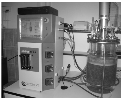
Fig. 1 – Laboratory-scale bioreactor for submerged cultivation of edible and medicinal mushrooms
