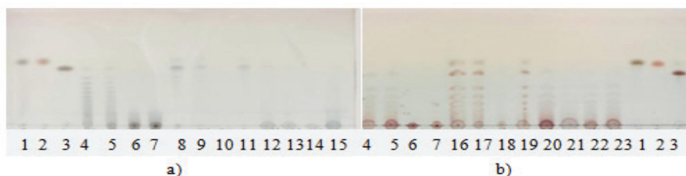
Figure 3. Thin-layer chromatography of fructans in 5 µl ethanol and 5 µl water extracts obtained from plants a) prickly lettuce ( Lactuca serriola L.) and b) annual sow thistle ( Sonchus oleraceus L.), standards 1-glucose, 2-fructose, 3-sucrose, 4 and 5-FOSs Frutafit CLR and HD, 6 and 7 - inulin Frutafit, TEX and Raftiline HP; 8, 9, 10, 11 – first, second, third and common ethanol extract from prickly lettuce; 12, 13, 14, 15 - first, second, third and common water extracts; 16,17,18 and 19 - first, second, third and common ethanol extracts; 20, 21, 22, 23 first, second, third and common water extracts from annual sow thistle.
